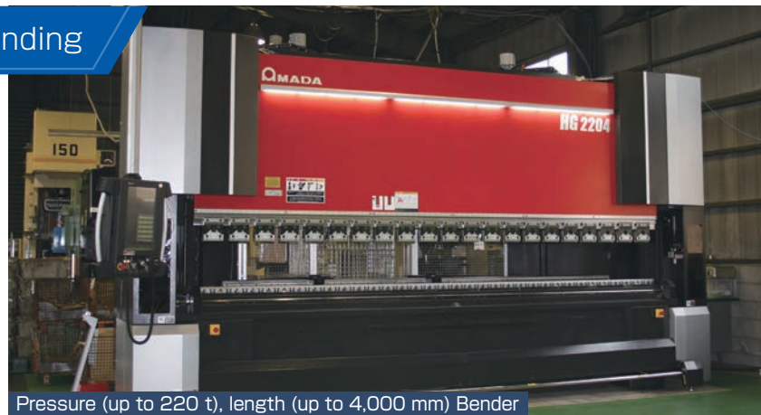
Pressure (up to 220 t), length (up to 4,000 mm) Bender
