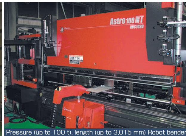
Pressure (up to 100 t), length (up to 3,015 mm) Robot bender
