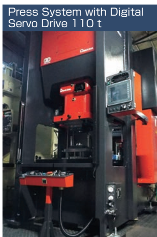
High speed and high accuracy press brake with dual servo press (DSP) drive mechanism
